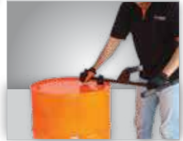
Removable handle used as a drum wrench
