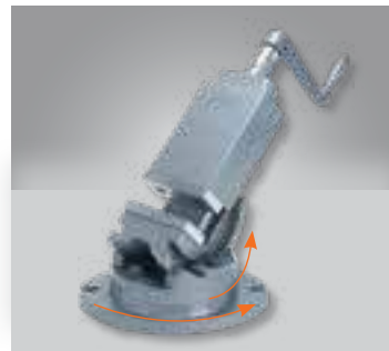
Combined rotation along both horizontal & vertical axis
