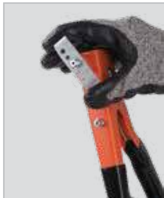
Convenient change of nose pieces with wrench
