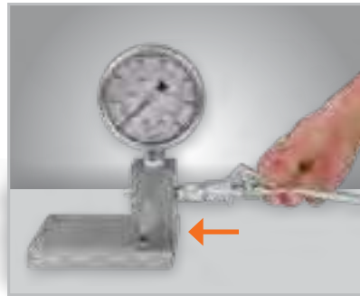
CONVENIENT ENGAGEMENT Press thumb lever and slide the coupler jaws on the grease fitting Coupler engages completely & remains firm thus allowing hands free operation
