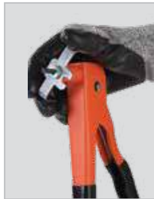
Convenient change of nose pieces with wrench
