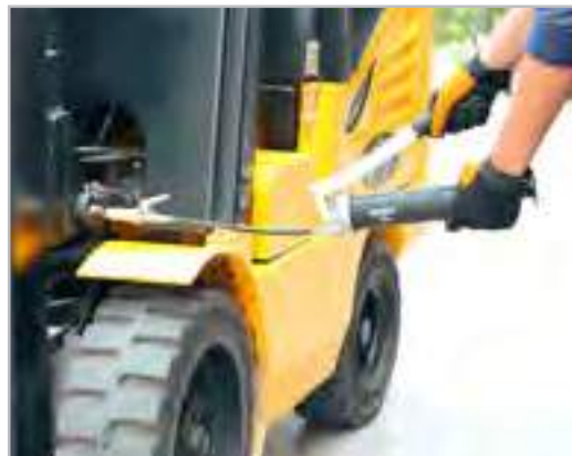
HANDS FREE OPERATION Coupler need not be held during greasing
