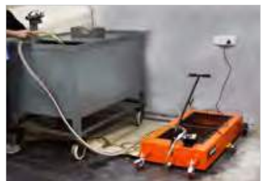
Extracting oil from the truck drain using AC power motor
