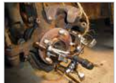
3 Jaw Puller used for removing tyre hub
